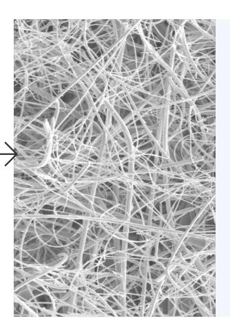
The AGM separators produced using purified water also exhibit exceptionally high purity, which can be clearly demonstrated in the SEM images.
