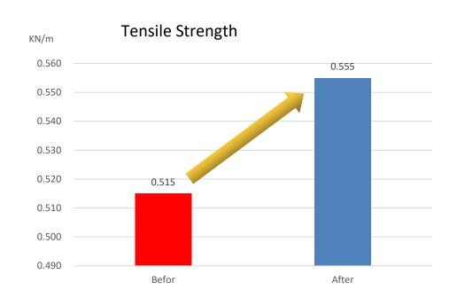
Under centralized intelligent control, the drying temperature is reduced while achieving optimized thermal profiles, preventing over-drying and aging of the glassfibers. This results in a significant improvement in the strength of the separators, and also resulting in significantly improved acid absorption with enhanced consistency.
