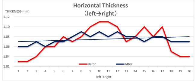
The formation system automatically modulates slice lip actuators based on real-time cross-direction (CD) basis weight and thickness profiles from online scanners, optimizing fiber pulp distribution uniformity and achieving grammage and thickness consistency.
