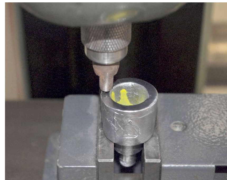
Vickers hardness tool and connector sample
