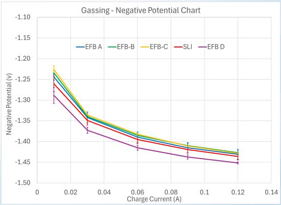
• The biggest difference in gassing is in negative potentials. EFB D negative shows more negative potential during the gassing test than others, which means it has the lowest gassing.
