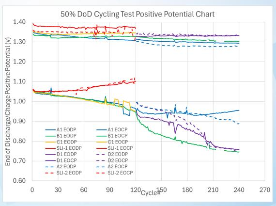
At 50% DoD cycling test, SLI and EFB A cells failed by negatives, EFB B, EFB C and EFB D failed by positives.
