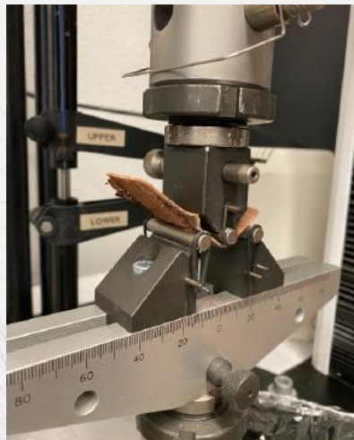
Mechanical testing of a lead battery using 3-point bend method.
