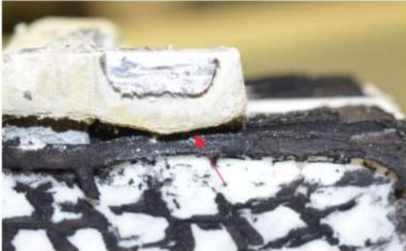
Positive grid growth leading to a connection with negative COS
